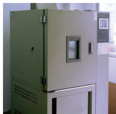
高低温湿热测试 High-low Temperature Damp Heat Test
