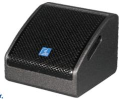
MR108 is a compact, small size, coaxial, 2-way full range monitor speaker, has balanced and real sound quality. Configuration:1x8" high efficency midbass unit and 1x1" exit throat 44mm voice coil HF driver with horn make up the coaxial. The cabinet is made of multilayer composite plywood with wear-resistant polyurea paint. MR108A is equipped with digital amplifier based on MR108 to be an active speaker.
