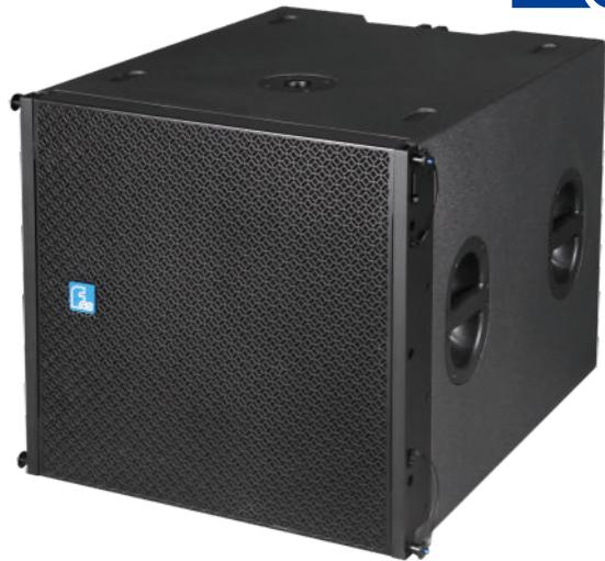
**DLA118B is a single 18" subwoofer.** It features 1x18" 100mm voice coil woofer, bass-reflex design, three-point hanging system matched with DLA408 and DLA112, can be hung and stacked to improve the low frequency performance of the system. The cabinet is made of multilayer composite plywood with wear-resistant polyurea paint. DLA118BAS is equipped with indepedant control two channels digital amplifier with DSP based on DLA118B to be an active system with DLA408 or DLA112.
